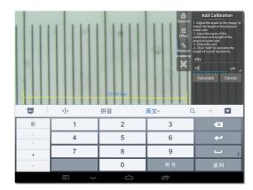
Enter the name for the calibration and actual length of the ruler. In the example, the name of the calibration is "40x", which corresponds to the magnification value of the chosen eyepiece, and "20µm" is the actual length of the chosen ruler.
